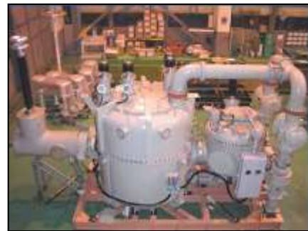
Fig. 9: 63 MVA/220 kV SF 6 power transformer.
