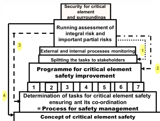
Fig. 6: Model of safety management of a critical element with automated control in time according to [11]. Processes: 1- conception and management; 2 - administrative procedures; 3 - technical matters; 4 - external cooperation; 5 - emergency preparedness; 6 - documentation and investigation of accidents; 7-
