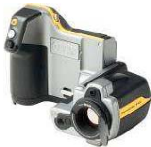
Figure 7: Infrared camera FLIR B335
