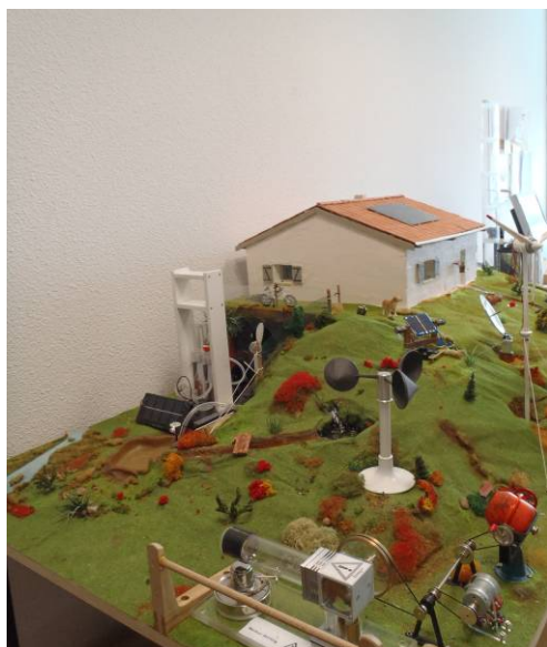
Figure 12: Global installation: Hydrogen cells, wind generator, mobile solar panel, Stirling engine, artificial river and pool.
