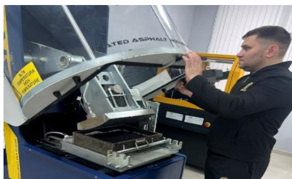
Fig. 5: Compacted slab specimen prepared for rutting testing. Source: created by the authors.
