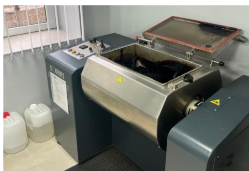
Fig. 4: Laboratory mixer used for the preparation of asphalt mixtures under controlled temperature and pressure. Source: created by the authors.
