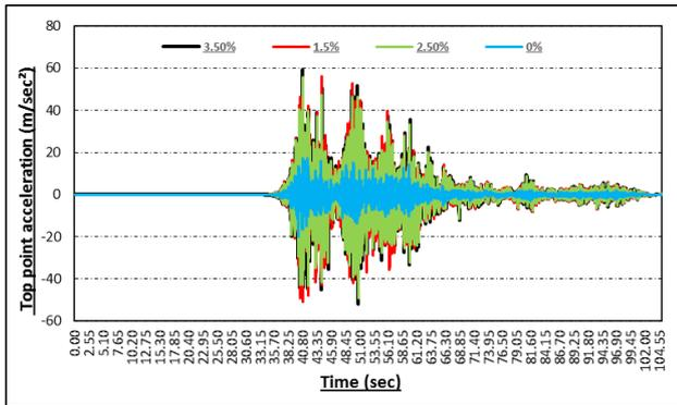
Fig. 4: Displacement accelerations of chimney top point
