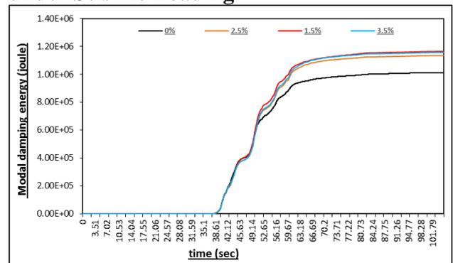
Fig. 7: Modal damping energies of chimney
