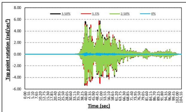
Fig. 5: Rotation accelerations of chimney top point
