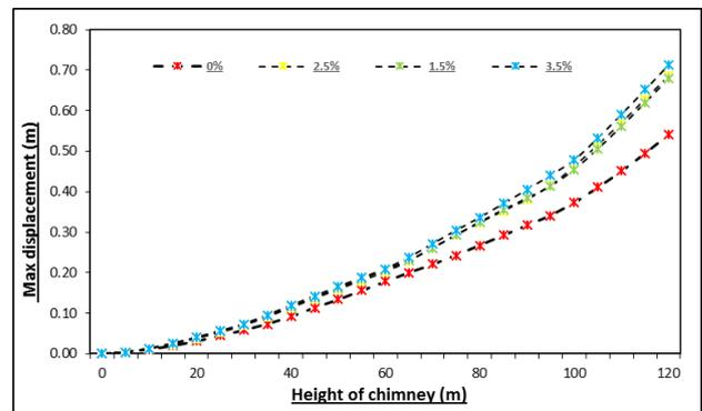
Fig. 6: Maximum displacements of chimney due to height
