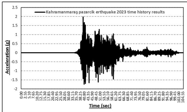
Fig. 2: Kahramanmaraş pazarcık earthquake 2023 recorded accelerations, [12]
