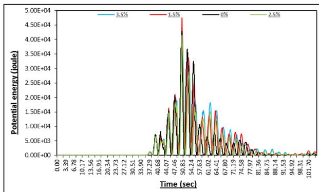
Fig. 11: Potential energies of chimney
