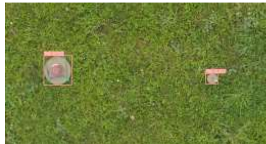
Fig. 1: Detected uncovered landmines in the optical image by CNN
