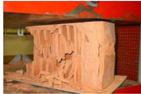
Fig. 4: Aspect of the final phase of the compression test
