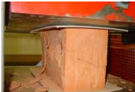
Fig. 2: Aspect of the intermediate phase of the compression test
