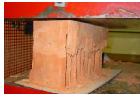
Fig. 5: Another aspect of the final phase of the compression test
