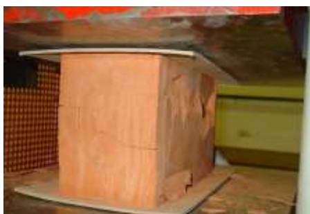
Fig. 3: Another aspect of the intermediate phase of the compression test
