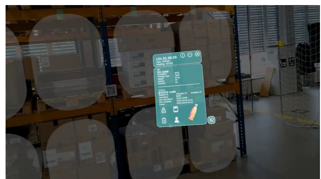
Figure 2: The storage inspection tool: in the foreground, the interaction menu; in the background, the shelves' selection grid
