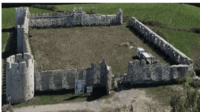
Fig. 6: Point Cloud generated from UAV Photogrammetry
