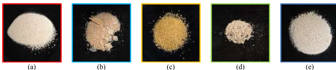
Fig. 6: Precipitated calcium carbonate: (a) P. mirabilis TISTR 100, (b) B. thuringiensis TISTR 126, (c) S. aureus TISTR 118, (d) Bacillus sp. TISTR 658, and (e) B. megaterium TISTR 067
