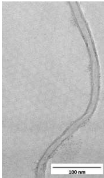
Fig. 9: TEM image of CNTs after purification by \text{HNO}_3
