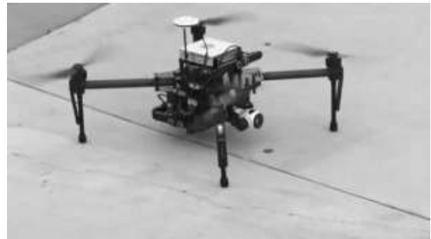
Fig. 1: UAV used for road inspection
