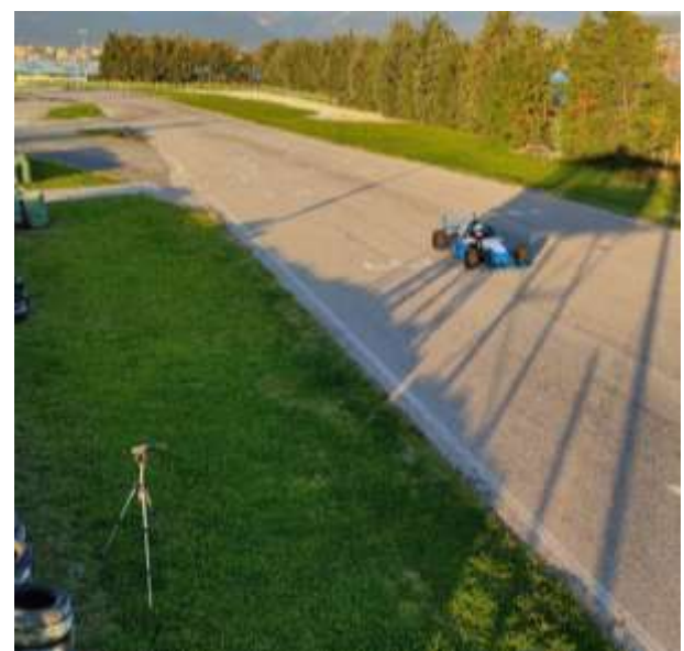
Fig. 3: Sound Level Meter position at point A during the single vehicle test.
