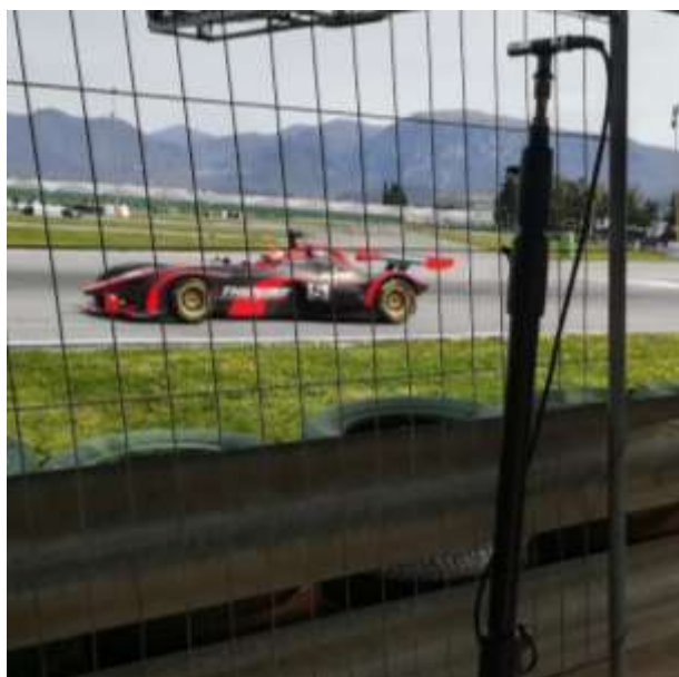
Fig. 4: Sound Level Meter position at point B during the race sessions.
