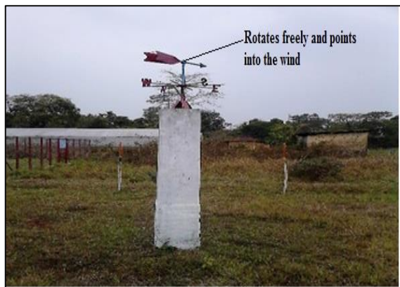
Fig. 7: Wind vane used for showing wind direction (Photograph: Khairuz Zaman)
