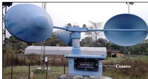
Fig. 3: Photographic view of cup counter anemometer (Photograph taken by: Khairuz Zaman)
