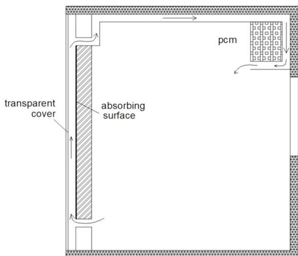
Figure 2 Cross-section with the pcm (case c)
