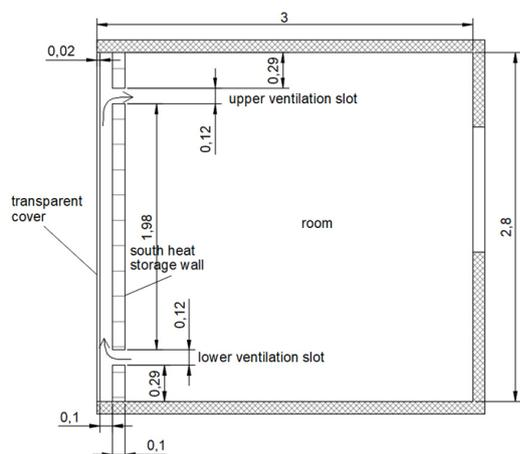
Figure 1 Cross-section of examined chamber without pcm (cases a and b)
