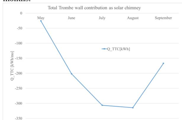
Figure 10. Total energy contribution from the Trombe wall,  $Q_{TTC}$  [kWh/mo]
