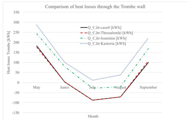
Figure 12. Heat losses through Trombe wall in the examined locations
