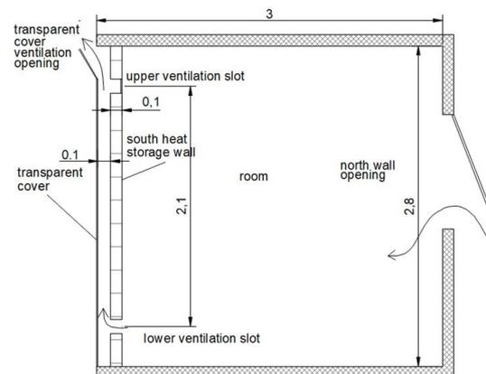
Figure 3. Cross-section for the solar chimney operation
