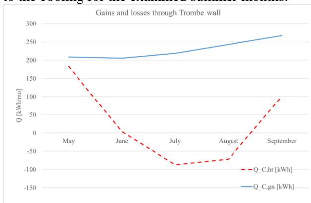
Figure 9. Cooling loads and cooling contribution from Trombe wall
