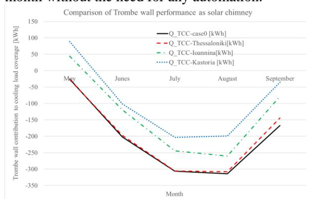
Figure 13. Comparison of Trombe wall performance as solar chimney in examined locations
