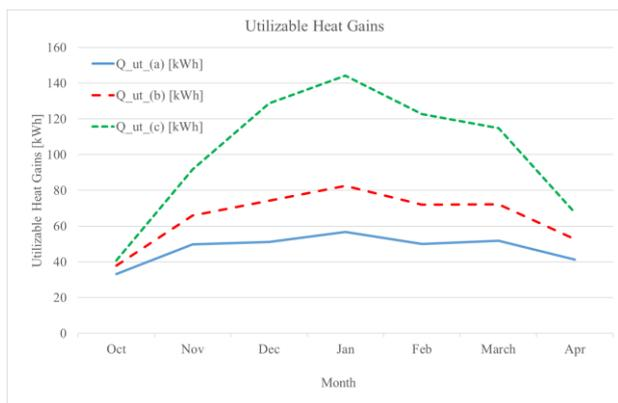
Figure 7. Trombe wall utilizable heat gains
