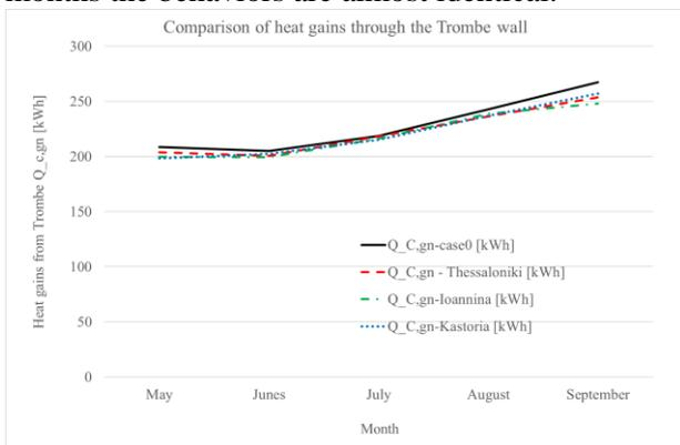
Figure 11. Heat gains from the Trombe in the examined locations
