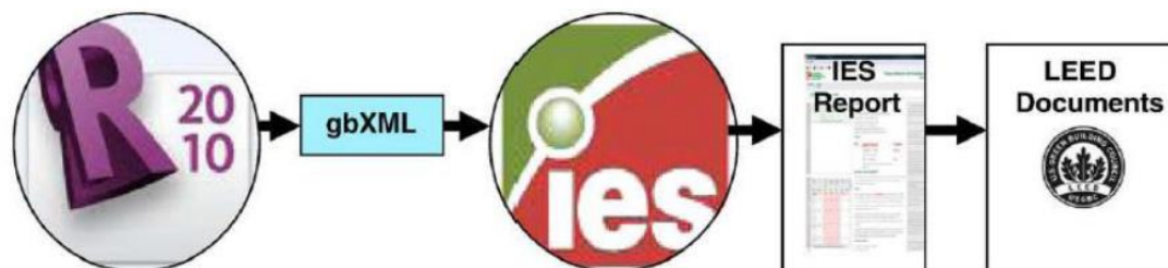
Fig.6: Key steps for sustainable analysis and LEED documentation using BIM and 3 rd party software.
