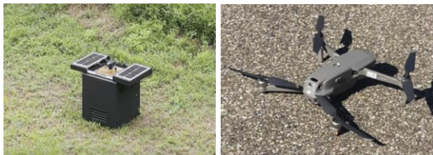
Figure 2 – UAV (a) and charging station (b).
