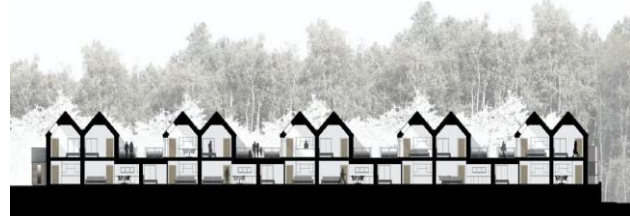
Figure (2) Section of the Tigh-Na-Cladach Housing Project [23]
