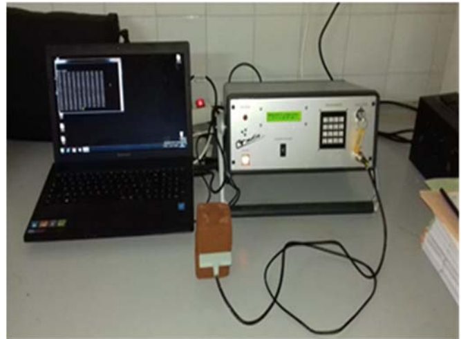
Fig. 1. General diagram of the <<CT-METRE>> allowing the measurement of the thermal conductivity of the samples
