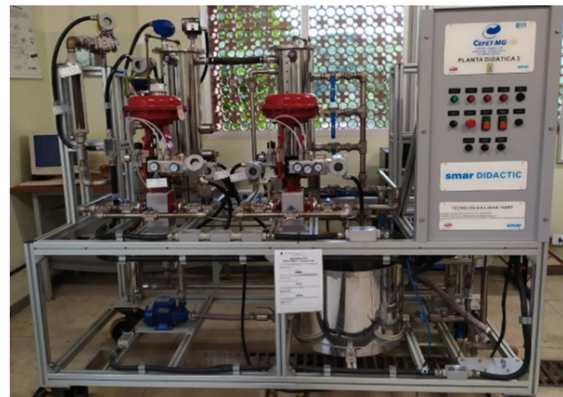
Figure 1: Didactic plant PD3 SMAR.
