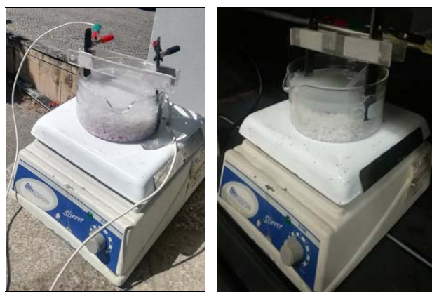
Fig. 3 UV radiation sources used for ATZ degradation in photoelectrocatalytic experiments: solar; UV lamp
