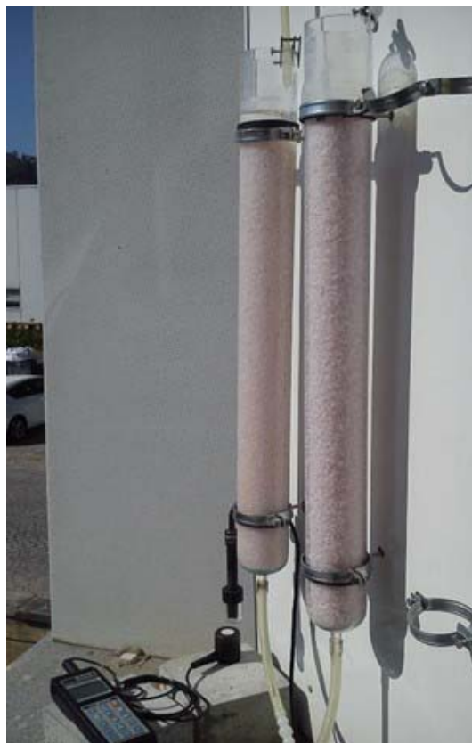
Fig. 2 Filtration columns with a quartz porous medium for OTC photo-oxidation (solar radiation)
