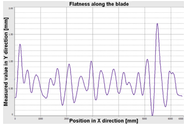
Fig. 16 The graph of flatness along the blade.
