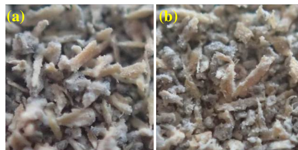
Fig. 7 Detail of particles with size 125 to 250 \mu\text{m} (a) cuttings crushed with jaws set at 6 mm; (b) cuttings crushed with jaws set at 10 mm
