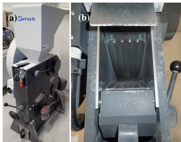
Fig. 2 (a) Jaw crusher (Retsch BB200 Mangan); (b) detail of the crusher jaws
