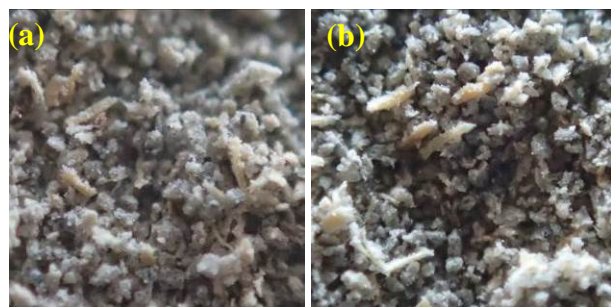
Fig. 6 Detail of particles with size 63 to 125 \mu\text{m} (a) cuttings crushed with jaws set at 6 mm; (b) cuttings crushed with jaws set at 10 mm
