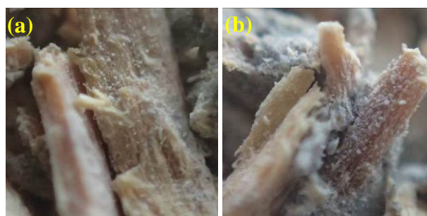
Fig. 9 Detail of particles with size 500 to 1,000 \mu\text{m} (a) cuttings crushed with jaws set at 6 mm; (b) cuttings crushed with jaws set at 10 mm
