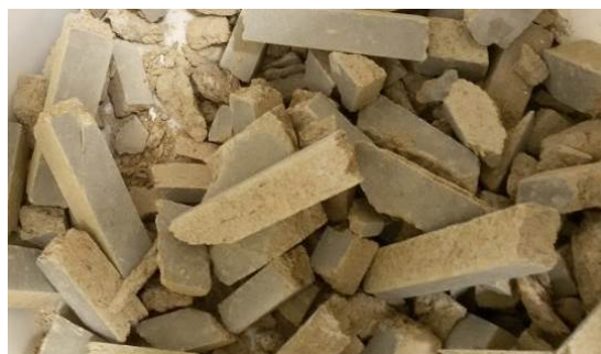
Fig. 1 Cuttings as a by-product from formatting cement-bonded particleboards during their production (producer – CIDEM Hranice, a.s.)
