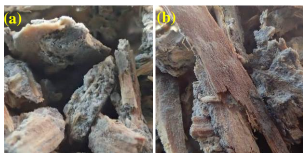
Fig. 11 Detail of particles with size 2 to 4 mm (a) cuttings crushed with jaws set at 6 mm; (b) cuttings crushed with jaws set at 10 mm
