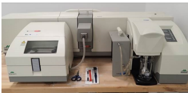
Fig. 3 Device for particle size distribution analysis (Malvern Mastersizer 2000E System EPA5011 including accessories)
