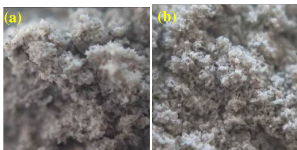
Fig. 5 Detail of particles with size 0 to 63 \mu\text{m} (a) cuttings crushed with jaws set at 6 mm; (b) cuttings crushed with jaws set at 10 mm
