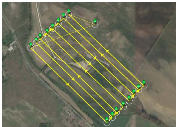
Fig. 1. The flight plan of the area, where recording is intended to take place (Mission Planner)
