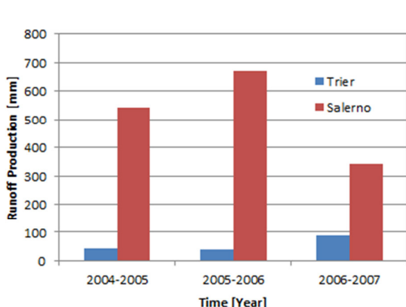
Fig.7:Green roof runoff production under Mediterranean (Salerno) and Oceanic (Trier) climate conditions
