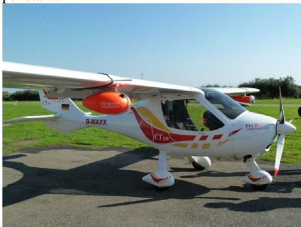
Figure 1: Research aircraft "Flight Design CT" with underwing measurement PODs
