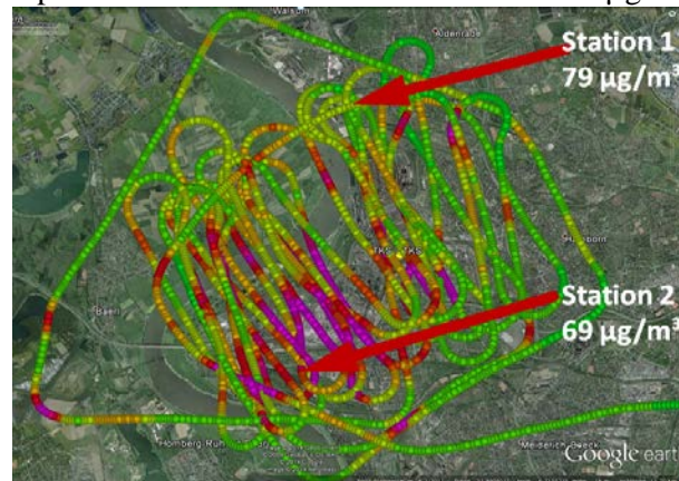
Fig. 8: Aircraft investigations of PM10 emission hot spots within the area of a steel company
