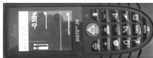
Fig. 2 - Reading gradient value with DISTO D83
