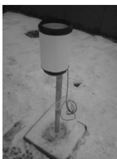
Fig. 2 rain gauge on the roof of University library [8]
