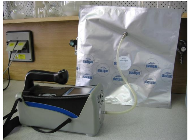
Fig. 6.: Measuring instrument ECOPROBE 5 – an example of calibration
