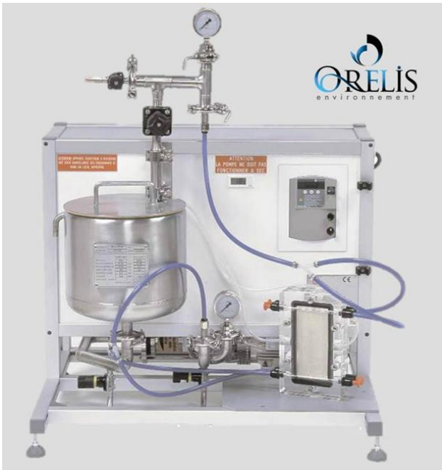
Fig. 5.: Real picture of experimental apparatus for MF/UF experiments
