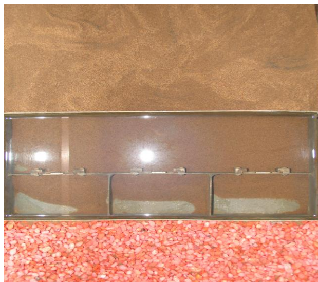
Fig. 2, A typical photo of measuring device (trap) for collecting interested sediment particles such as fine sand (shown above), course sand, very course sand, and fine grain
