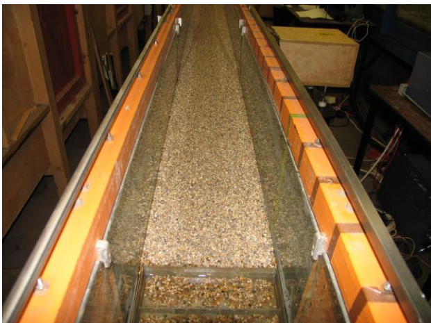
Fig. 11, A typical photo of the bedform obtained for a bed with very course sand water worked
