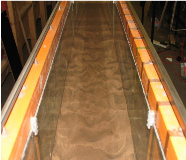
Fig. 7, A typical photo of the bedform obtained for bed with very fine sand water worked
