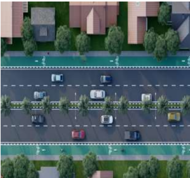
Figure 5. Protected Bicycle Lane General Design Proposal
