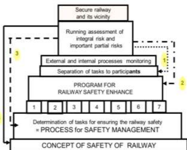
Fig. 1. Railway CSMS model with automated control over time. Processes: 1- conception and management; 2 - administrative procedures; 3 - technical processes; 4 - external cooperation; 5 - emergency readiness; 6 - documentation and investigation of accidents; 7- cybersecurity. Feedbacks: 1-4 in yellow circles- processed according to [32].
