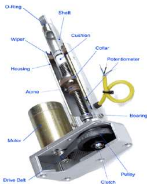
Fig. 3: Linear actuator, [6]
