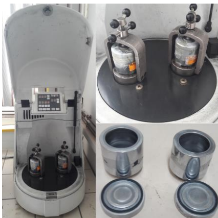
Fig.1. Pulversiette 7 planetary ball mill and vials used in experiment.
