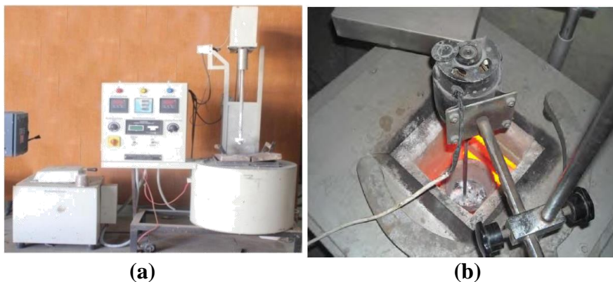
Figure 4: (a) Stir Casting and (b) Electrical Furnace Equipment
