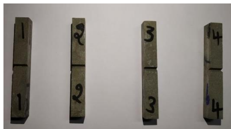
Figure 9: Impact test specimens as per ASTM E8M04 standards.
