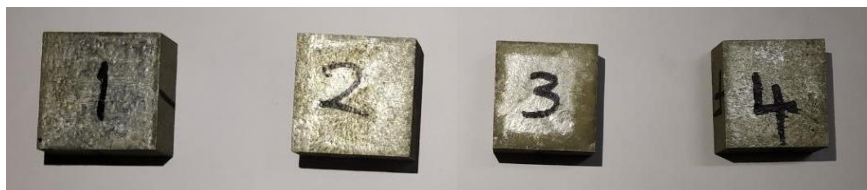
Figure 13: Impact test specimens as per ASTM E8M04 standards.
