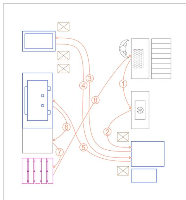
between each operation that a worker must complete to accomplish the complete assembly process. The assembly process paths are marked in sequence, following the established assembly sequence.
