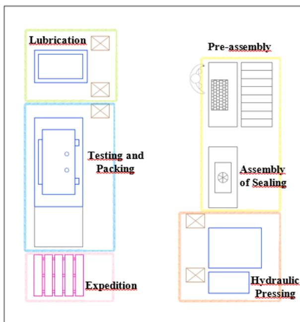
Fig. 2 Layout of the Assembly Workplace
