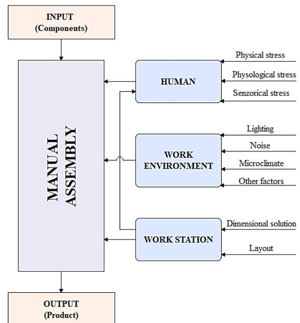
Fig. 1 Elements of a Working System [12]
