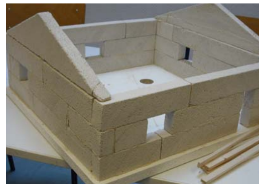
Figure 2: AAC external walls building
