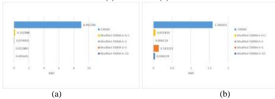
Fig. 3: The RMI values of the EWMA and modified EWMA control charts for example 1 when (a) \lambda = 0.05 and (b) \lambda = 0.10
