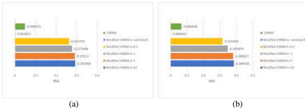
Fig. 4: The RMI values of the EWMA and modified EWMA control charts for example 2 when (a) \lambda = 0.05 and (b) \lambda = 0.10
