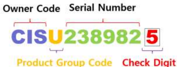
Fig. 3: Container BIC Code Structure
