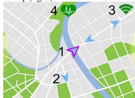
Fig. 3. Visual interface. 1 – current position; 2 – other vehicle; 3 – server connection indicator; 4 – driver’s state indicator.
