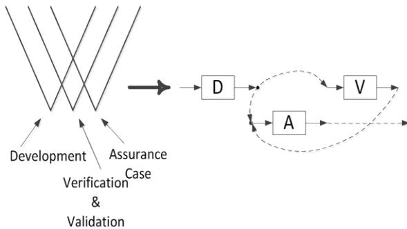
Fig.12. Transition from V-shape Life Cycle to Development-V&V-Assurance Case (DVA) Notation
