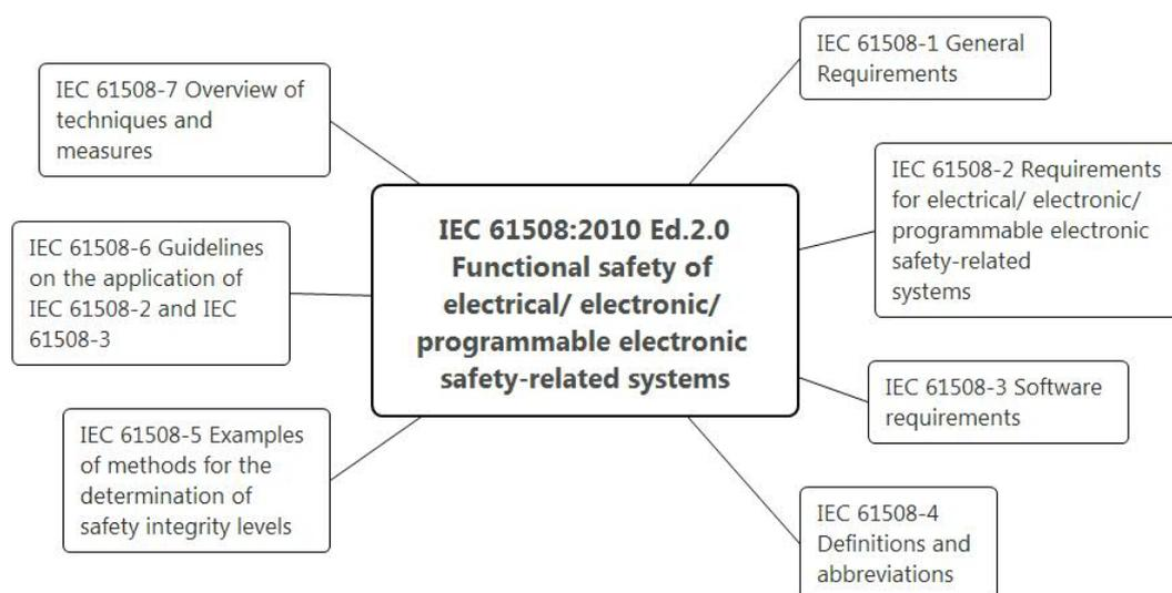
Fig.5. A Structure of the Standards Series IEC 61508
