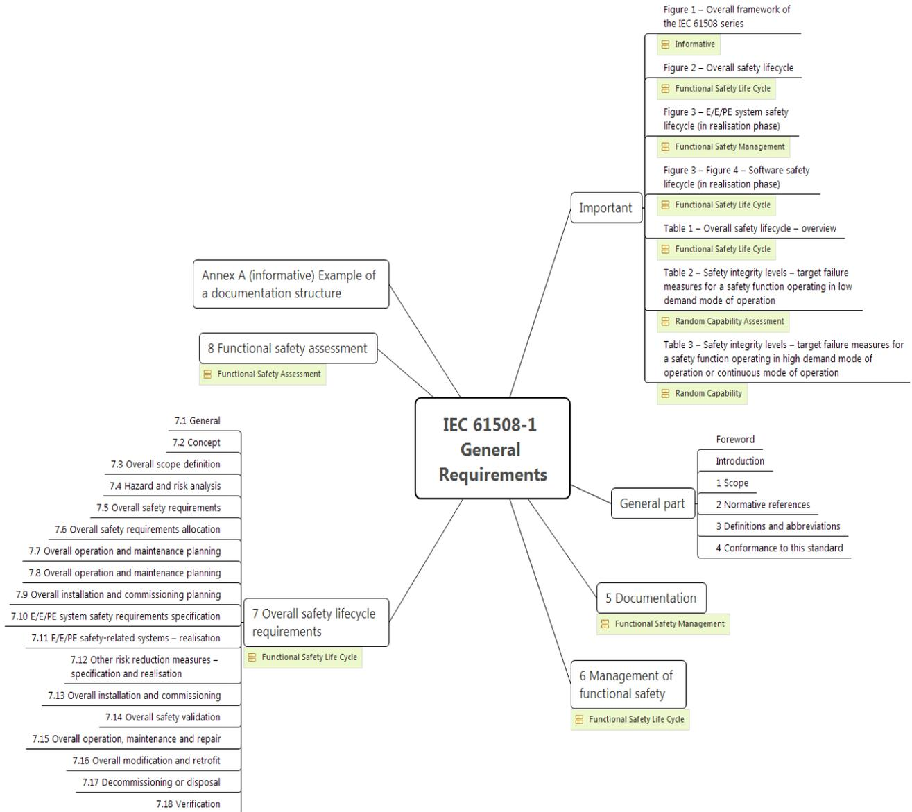
Fig.8. Structure of the Standard IEC 61508 – Part 1: General Requirements
