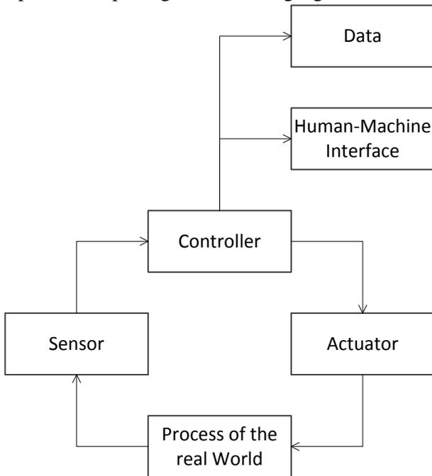
Fig.2. Typical Architecture of Computer Control Systems
