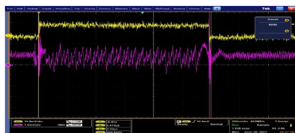
Fig. 11: Power leakage traces of GIFT-128 Source: Created by the authors
