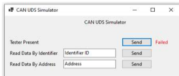
Fig. 11: Negative results for the "Tester Present" test
