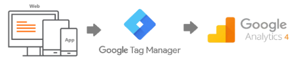
Fig. 1: Collecting data from the Web and app with GTM and sending to GA4
