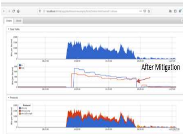
Fig. 10: flow After mitigation of TCP traffic
