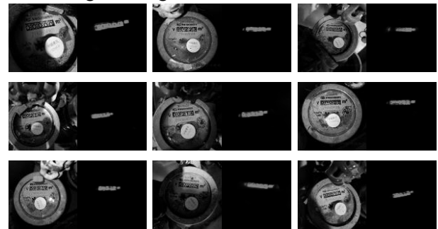
Fig.7 Pretreatment images of water meter (left) and reading area segmentation result (right)
