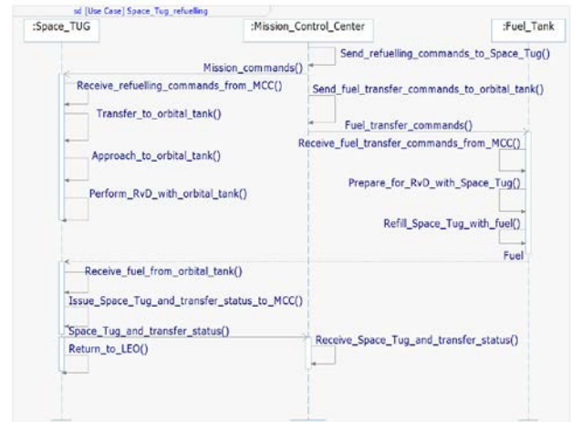
Figure 8: Sequence Diagram describing the Space Tug refuelling phase
