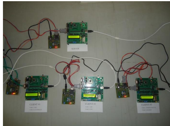
Figure 3: A close view of LPC2148 Microcontroller based Multiprocessor System
