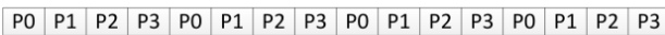
Fig. 4. Optimal memory storage layout for 4 particles of 4D resulting in a coalescing memory access pattern to global memory
